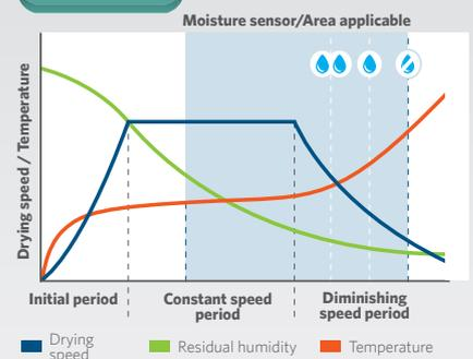
The residual moisture control system is highly accurate and reliable. Prevents the linen from overdrying and shortens the cycle time.
