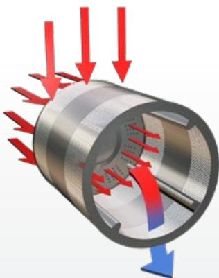
Directing the flow of air through the linen and making the most of their temperature are key factors in getting the best performance from a dryer.
