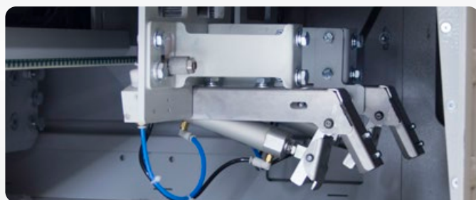
New server clamps, more robust for heavy articles
