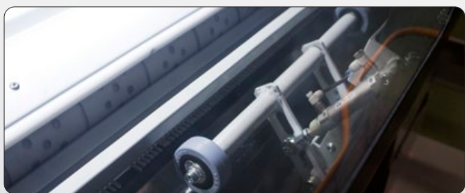
A system of compressing rollers during feeding to ensure that the item is loaded correctly, especially if it is heavy or has a tendency to slide.
